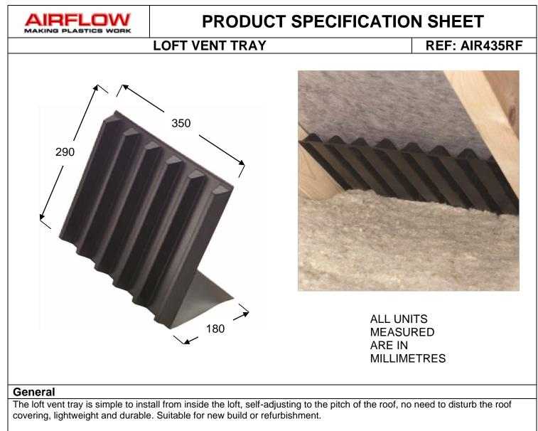
To install, just flex the tray at the crease and position it into the eaves between the rafters from inside the loft, making sure the ridges face the towards the underlay. You need to push the insulation up to the tray to hold it in place and check that the insulation material does not touch the roofing underlay. If you need wider spacing the trays can be clipped together to provide 10mm airflow
